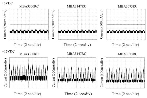
Figure 4.7 shows the Max Seek current waveform of +5V DC and +12V DC.
